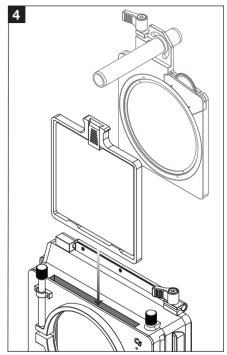
4. Insert the C501-103A or C5 VND into the mounting slot on the top of C5 matte box.
