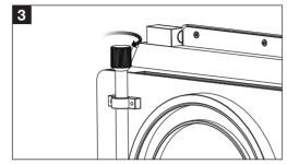
3. Tighten the adapter ring locking screw clockwise to clamp the adapter ring on to the C5 matte box.
