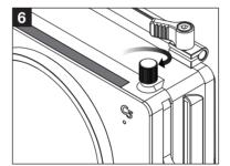
6. Tighten the locking screw for the mounting slot of C501-102A. This locks it securely to the C5 matte box.
