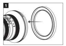
1. Select the adapter ring that fits the lens diameter, and tighten the adapter ring clockwise on the lens.
